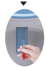
Step 2 Fully automatic aspiration and dilution procedures
